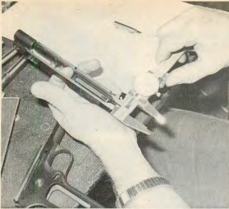
Above: "Combat Accuracy Job" entailed precision making of frame, slide, and barrel. Here, Starks mikes inside dimensions of grooves in .45 Combat Commander slide.
